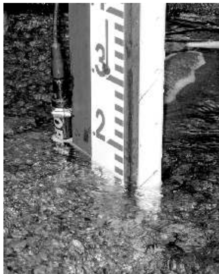
Figure 1. Left: A turbidity sensor installed in a natural stream channel. The OBS-3 probe was originally installed to specifications (D&A Instrument Company 1993), but a peak flow event changed the channel (as shown) and subsequently forced the relocation of this station. Right: An Analite 9500 turbidity probe set up in a laboratory. This brand of probe has a smaller "viewing window," which enables it to measure turbidity in a more confined environment.
